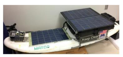
Figure 1. MARCo autonomous unmanned surface vehicle.
